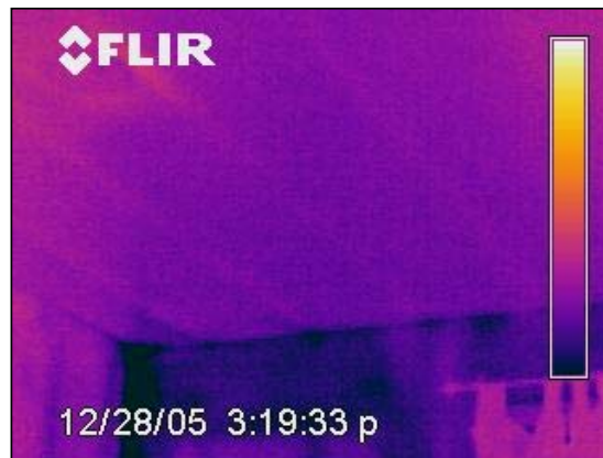
Figure 14.2 - Cold air infiltration into home via porch roof
