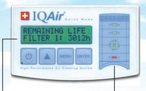
**Intelligent Filter Life Monitor** Tracks life of each individual filter to maximize performance and yield. Calculates remaining filter life down to the hour, based on actual usage.
