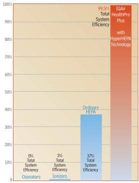
Total System Efficiency (Particle Retention) for Particle Sizes: 0.01 - 1.00 microns
